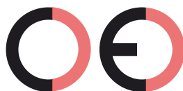
False CE Mark (too far)
